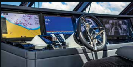
LEFT Paragon's glass bridge is dominated by four 19-inch Raymarine Axiom displays.
